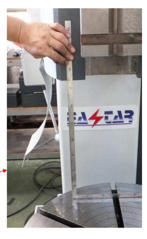
While Max. stroke: 300mm, the distance form the ram end to rotary table is 460mm.
